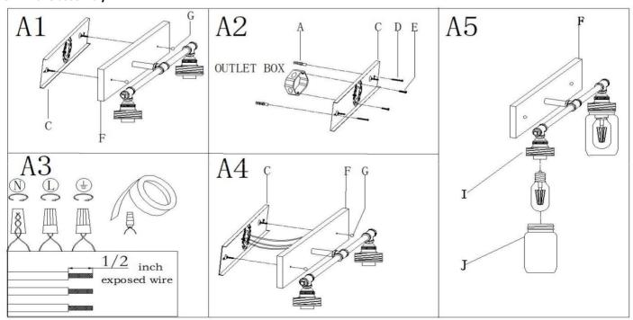
Step A1: Unscrew the ball knobs(G) from the back plate(F) then gently remove the mounting plate (C)
