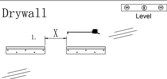
1>Put the hanging cleat on the wall, confirm the position of the hanging cleat, and level the hook with a level ruler
