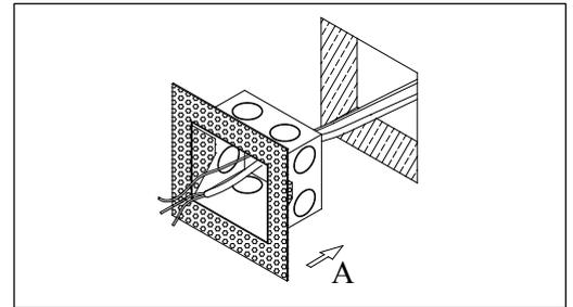
Step.1: Fix the Mounting box(B) to the hole.
