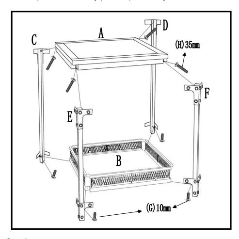
**Step 1**Attach the Legs (C) (D) (E) (F) to the Shelf (B), use Allen Key to tighten the Bolts (G) Then put the Top (A) on to the Legs, tighten the Bolts (H)
