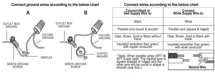
Twist wires together with plastic wire connectors until tightly joined.
