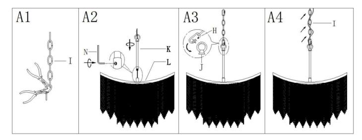
Step A1 » By measuring, determine the correct number of links needed for proper hanging height. Using the chain pliers, disconnect and discard the unwanted part.
