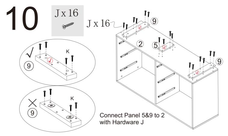
**ATTENTION**: When you assemble the part 5/9 to the board 2 and see the  $\sqrt{10}$  facing your face, that means the direction of the part 5/9 is right.
