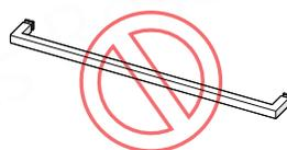
**DO NOT** attach the Handle to the Door Glass until instructed. **DO NOT** use the handle to lift the glass during installation. This may result in damage to the glass and/or serious personal injury. Always use an assistant and/or a professional-grade glass suction cup when handling heavy glass panels.
