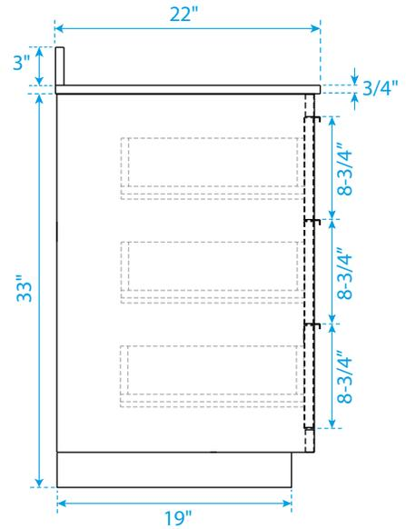
\*Note: Due to high probability of breakage, the backsplash comes in two pieces, cut from the same piece. All measurements are  $\pm 1/4"$ .
