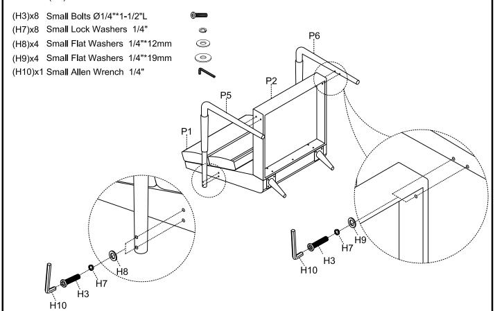
**Step 4.** a) Securely tighten all bolts with Allen wrench(H6&H10), turn the assembled chair to an upright position. b) Insert the wooden plugs (H11) to the arm with Legs (P5&P6) as shown below. Failure to follow these instructions may cause the bolts to misalign during assembly. Assembly is complete.
