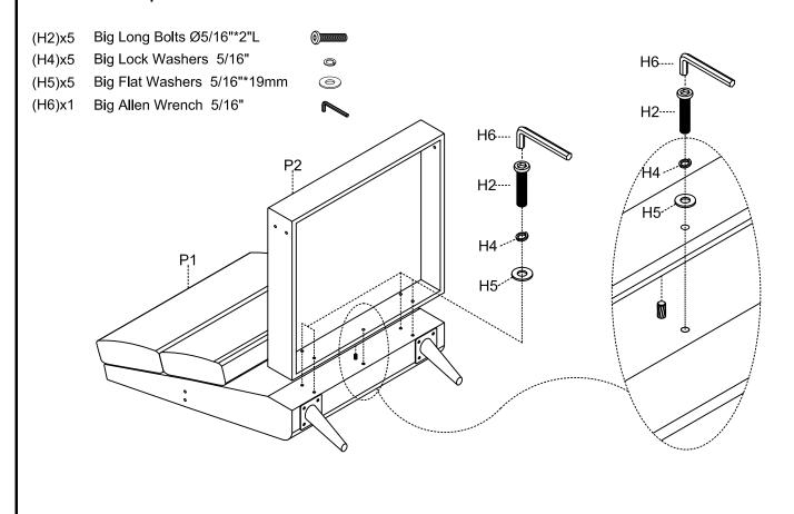
**Step 3.** Attach left arm with Leg (P5) and right arm with Leg (P4) to the assembled seat frame (P2) and back cushion (P1) as shown below.
