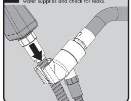
Ensure Hose Washer is inserted inside connector to avoid leaks. Thread Hose End with Label to the outlet port of Bracket. Hand tighten.
