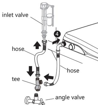
Normally, the tee is installed on the angle valve
