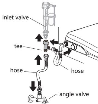
if the angle valve and wall is too close, you can install the tee under the inlet valve
