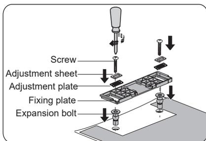
3. ① Insert the expansion bolt into ceramic hole;
