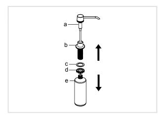
Install dispenser base (b) with washer attached into the hole in the countertop. Re-install washer (c) and mounting nut (d) on the dispenser base (b) from underneat countertop. Tighten mounting nut (d) by hand.
