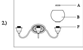
Step 2: Use the socket ring (A) to secure glass (B)on socket (F).
