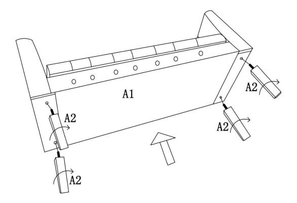
Attach Legs A2 to the bottom of Top Seat A1 as shown above.
