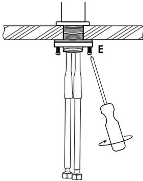
Slide washer and thread the mounting nut onto threaded shroud. Turn faucet to desired handle position. Securely tighten clamp screws (E)
