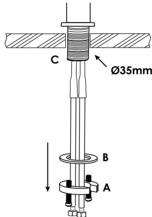
Ensure there is a Ø35mm through-hole on the kitchen counter. Remove the mounting nut (A) and washer (B) from the threaded shroud (C).
