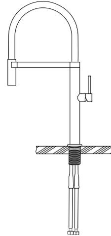
Position faucet on the installation surface. Fit flexible hoses through hole on countertop or sink.
