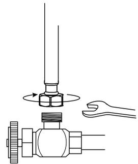
Connect hot and cold water lines to the inlet pipe and tighten with a wrench until snug. Do not over tight.
