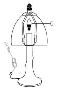
Step2 Insert the bulb(G) into the socket(C).
