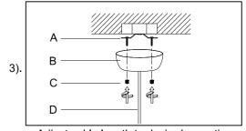
Step.3: Adjust cable length to desired mounting height, and tighten strain relief screws to secure. Install body (D) to bracket (A) and tighten finials (C) on the canopy (B) to secure.
