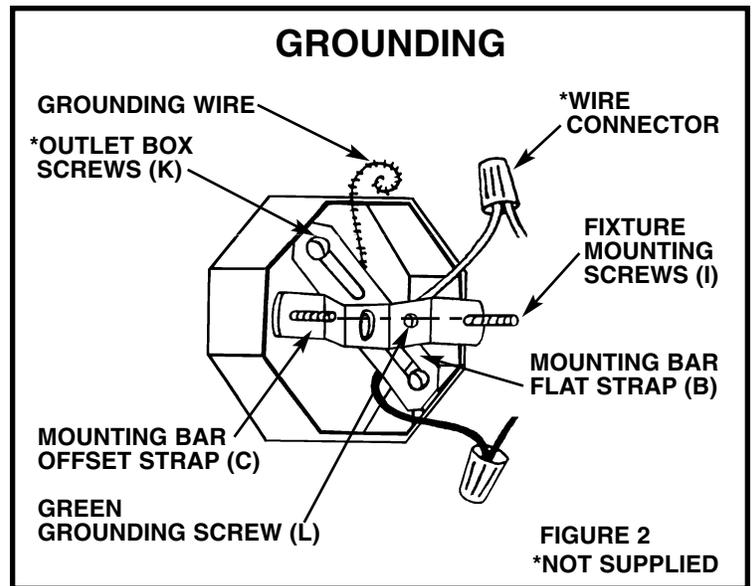
**WARNING: TO REDUCE THE RISK OF FIRE, ELECTRIC SHOCK OR PERSONAL INJURY, MOUNT TO OUTLET BOX OR SUPPORTING SYSTEM ABLE TO SUPPORT THE WEIGHT OF THE FIXTURE.**
