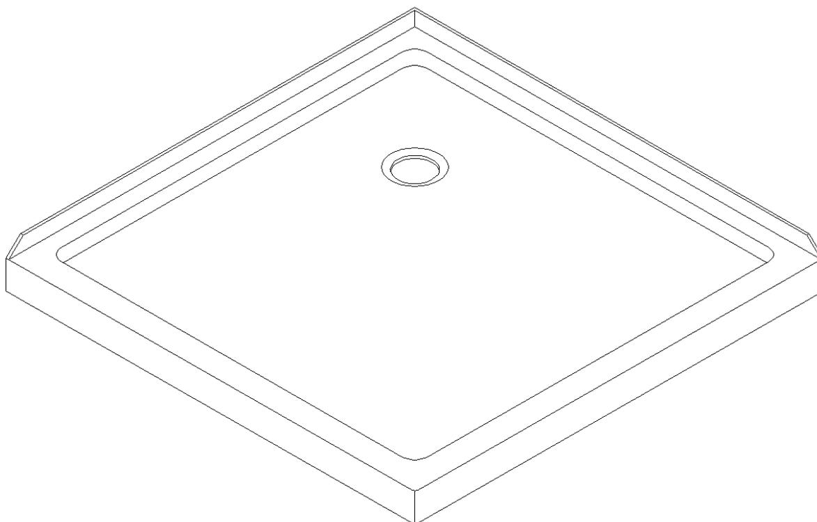
Double Threshold Shower Base with Corner Drain Configuration
