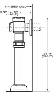
\*Note: The Critical Line (-C-L-) on Vacuum Breaker must typically be 6" (152mm) minimum above fixture. Consult Codes for details.
