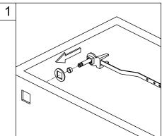
1. Insert plastic washer and flush arm through bracket, then place rubber washer onto bracket.
