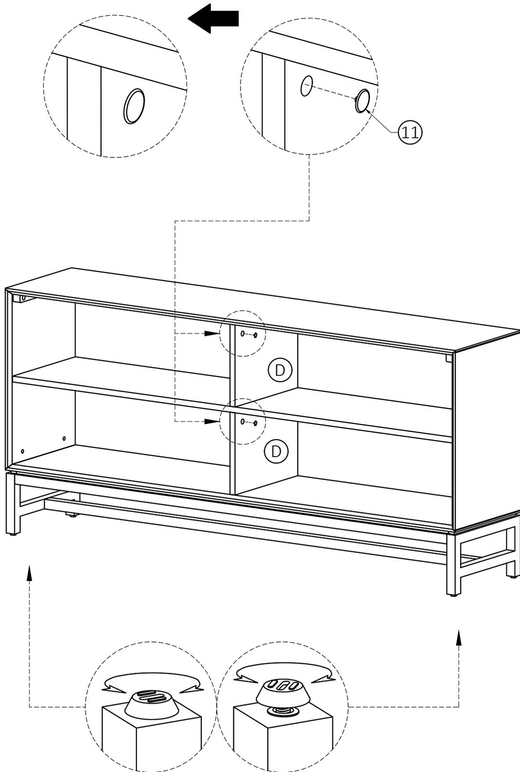
1. Insert four Plastic Caps (11) into holes Cam Locks on Dividers (D).
