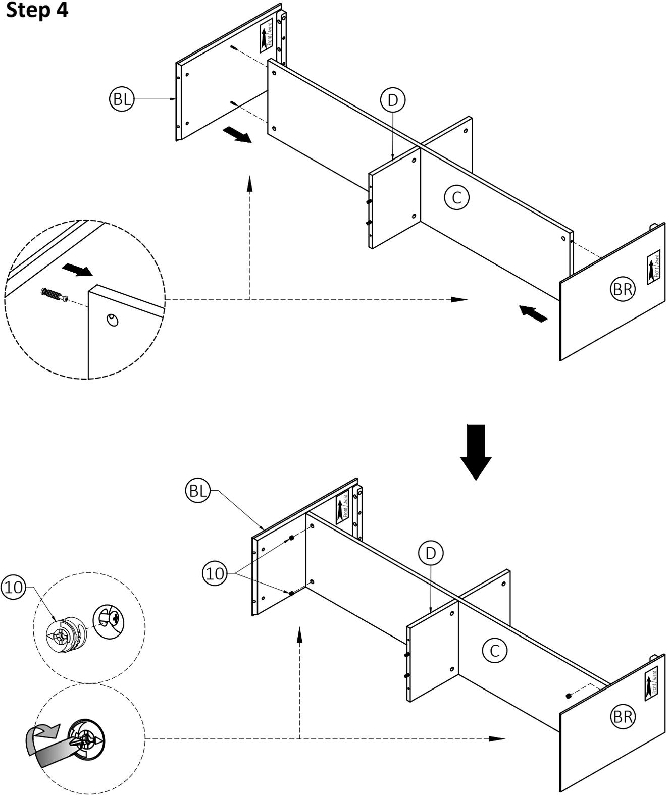
1. Align Cam Lock Pins with guide holes on Cabinet Shelf (C) and attach Sides (BL), (BR) to Cabinet Shelf (C).
