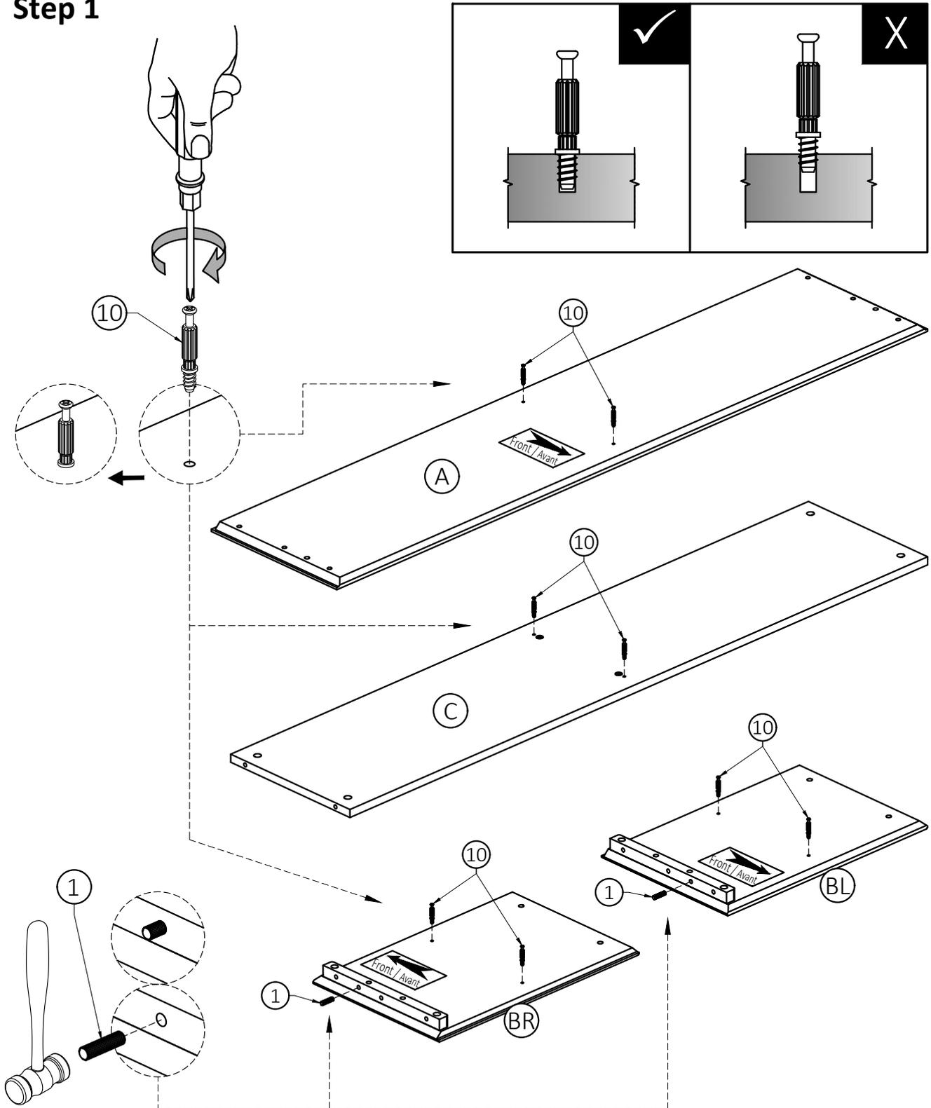
1. Attach Cam Lock Pins ⑩ into pre-drilled holes at Top ①, Cabinet Shelf ② and Sides ③, ④.
