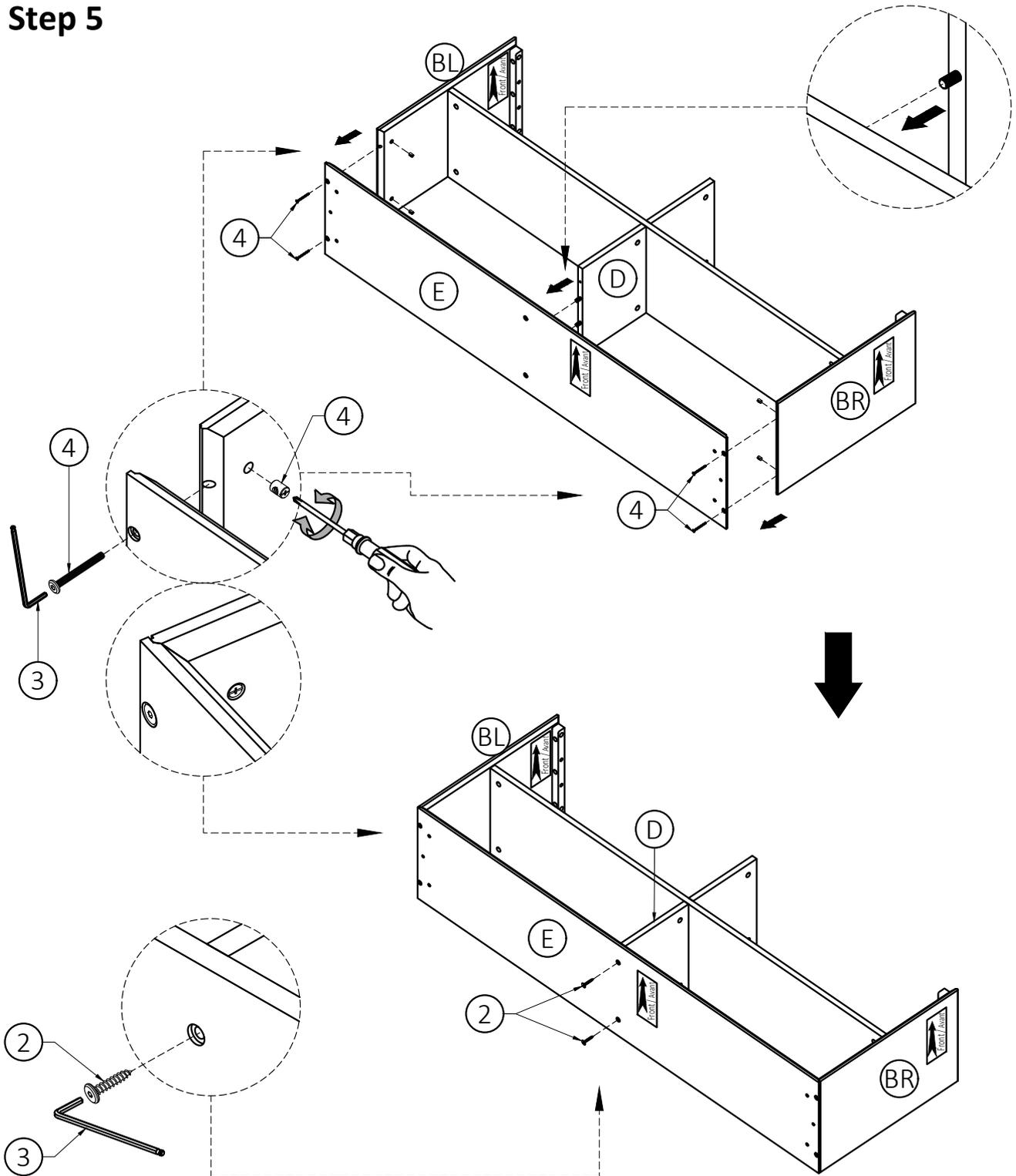
1. Align Wood Dowels with guide holes and attach Divider (D) to Bottom Shelf (E).
