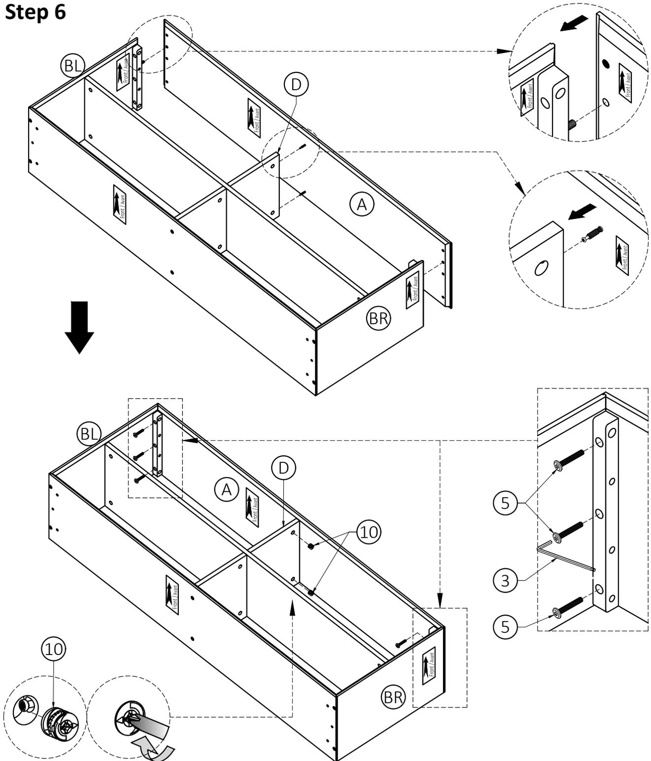
1. Align Wood Dowels and Cam Lock Pins with guide holes on Top (A) and attach Top (A) to Sides (BL), (BR) and Divider (D).
