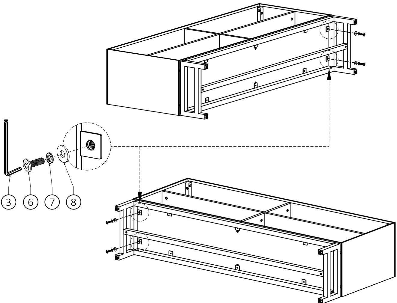
2. Use four Bolts (6), four Lock Washers (7) and four Washers (8) to secure metal frame and wooden frame .
