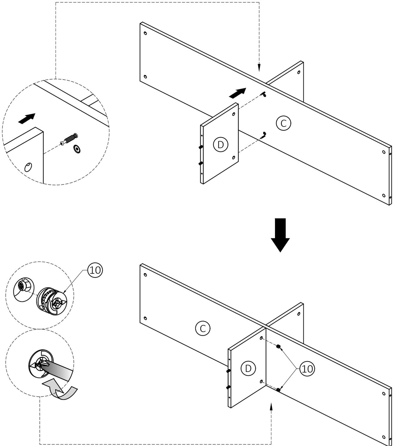
1. Align Cam Lock Pins with guide holes on Divider (D) and attach Divider (D) to Cabinet Shelf (C).
