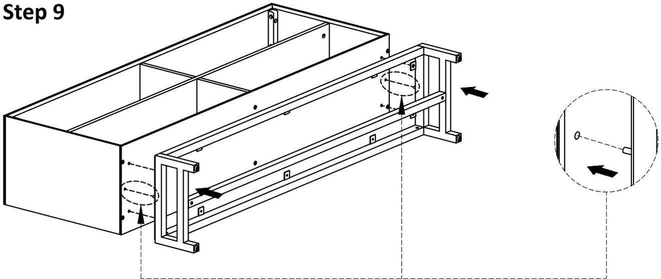
1. Align iron dowels with guide holes on wooden frame and attach the assembled metal frame to bottom wooden frame .
