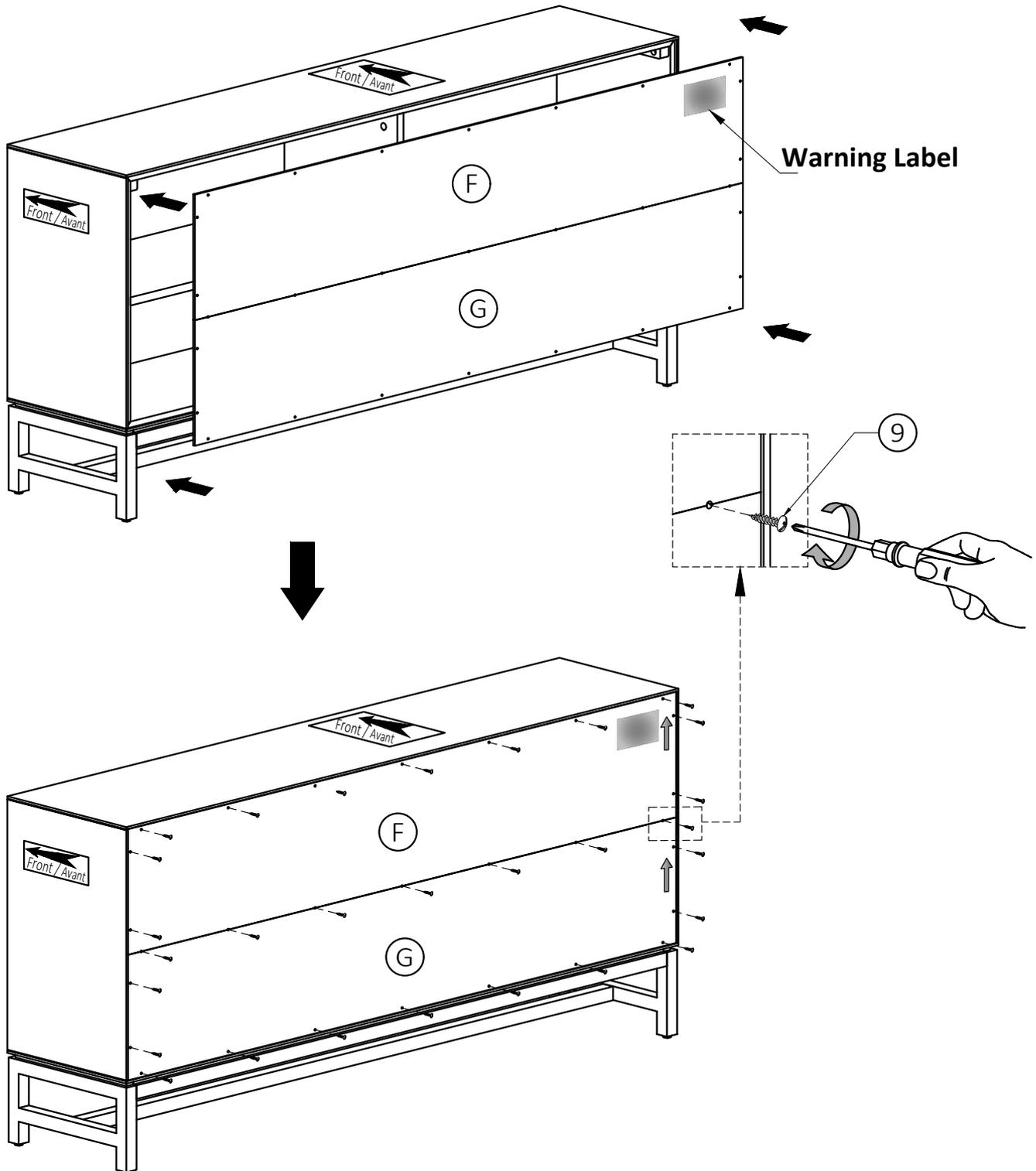
1. Attach the Back Panels (F)(G) to back frame using Phillips Screws Round Head (9) through guide holes from Back Panels.
