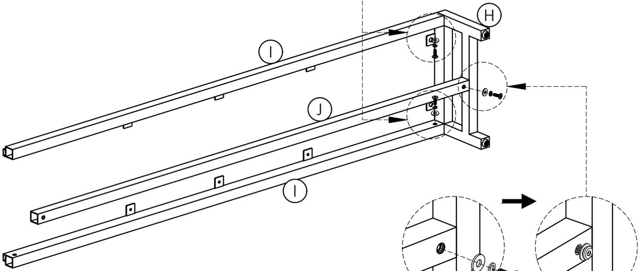
2. Use one Bolt (6), one Lock Washer (7) and one Washer (8) to secure each part (I),(J) with (H).
