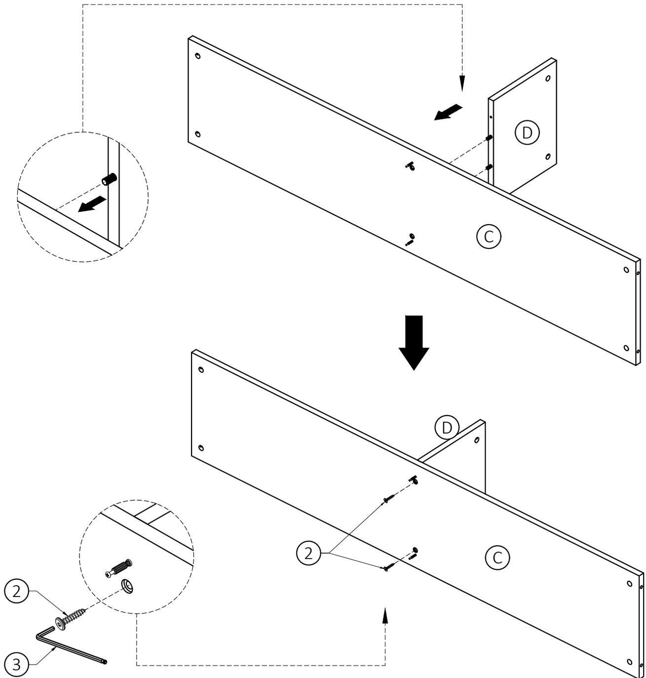
1. Align Wood Dowels with guide holes on Cabinet Shelf (C) and attach Divider (D) to Cabinet Shelf (C).
