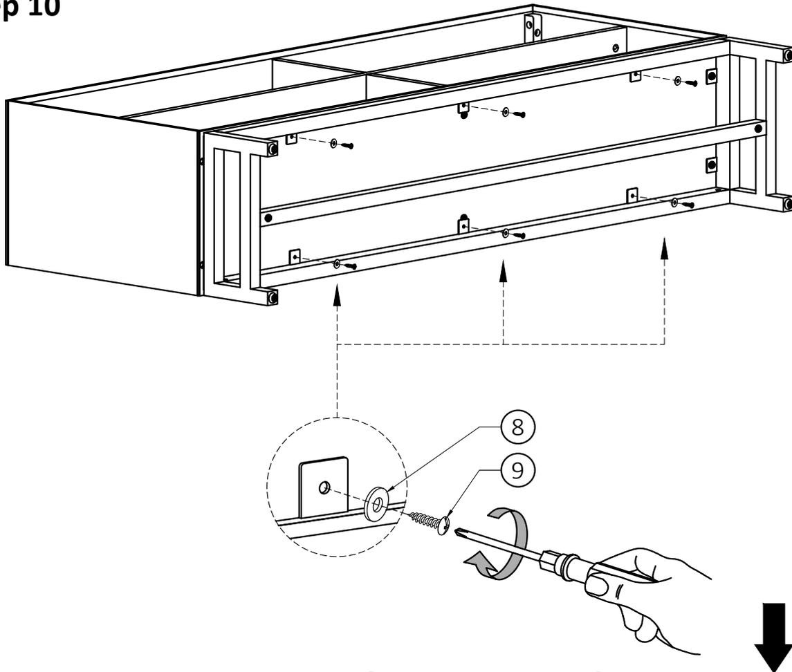
1. Use six Phillips Screws Round Head ⑨ and four Washers ⑧ to secure wooden frame and metal frame.
