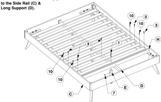
Bolt & screw the remaining Bed Slats (H) to the Side Rail (C).
