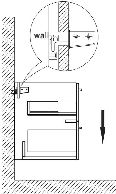
**4** Adjust the mounting attachment as required
