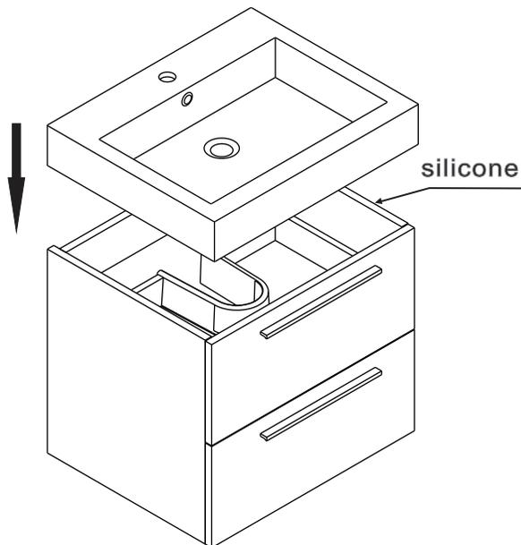
**6** Licensed professional installation is recommended. These instructions are for mounting into studs or other in-wall reinforcement, drywall alone is not sufficient to support wall-hung vanities. Other installation techniques may require a licensed professional.
