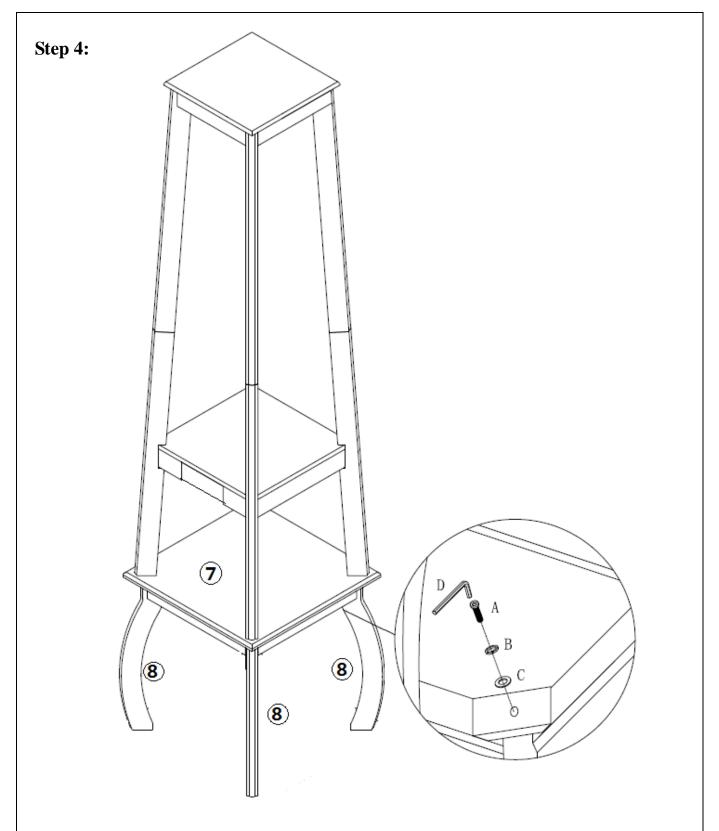
Assemble Bottom Posts (8) to Shelf (7) using Bolts (A) with Spring Washers (B)& Flat Washers (C) by Allen Wrench.
