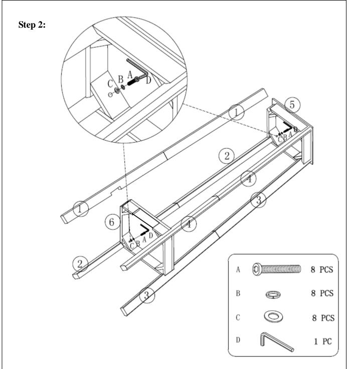
Assemble Posts (1), (2), (3), (4) to Top Panel (5) and Shelf w/Drawer (6) using Bolts (A) with Spring Washers (B) & Flat Washers (C) by Allen Wrench (D).
