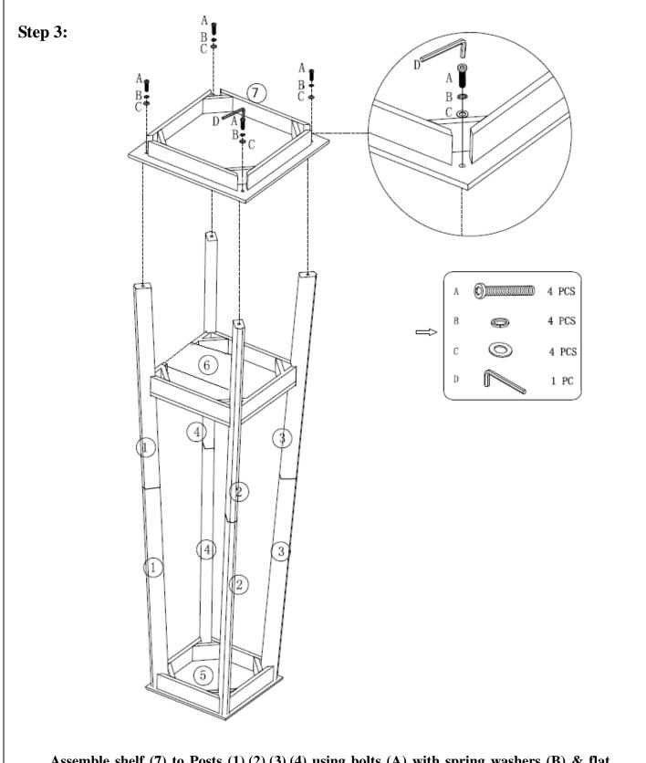
Assemble shelf (7) to Posts (1),(2),(3),(4) using bolts (A) with spring washers (B) & flat washers(C) by Allen Wrench.
