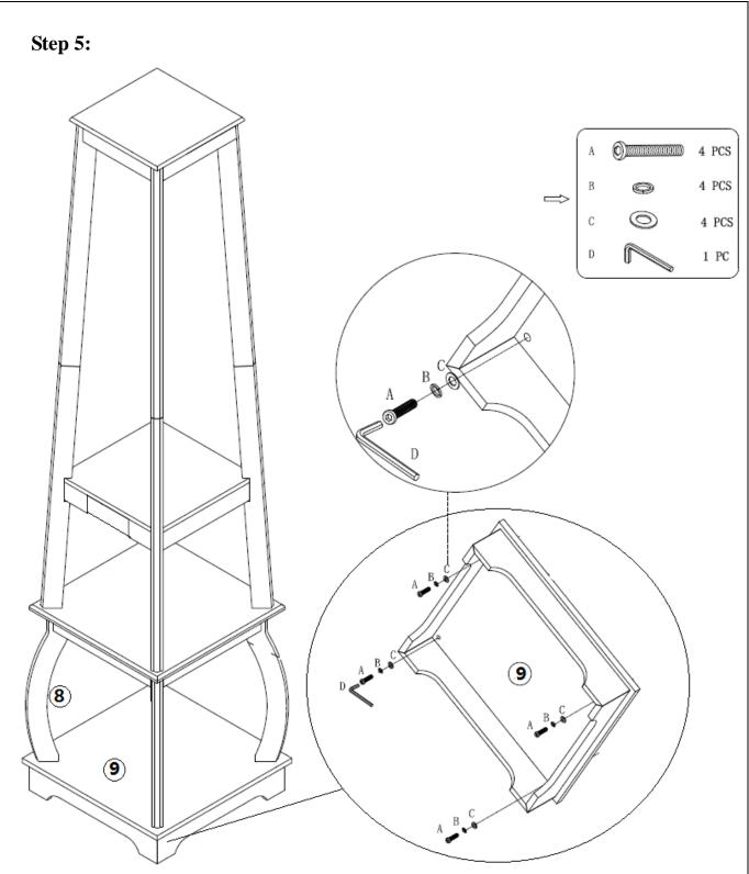
Assemble the Bottom Panel (9) to Bottom Legs (8) using Bolts (A) with Spring Washer(B) and Flat Washers (C).
