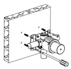
Install the valve body. Wrap the threaded portion of the joints in Teflon tape and connect the water inlet and outlet.
