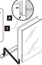
With assistance, rest the cabinet on the mounting bracket (I) and fold it in place.
