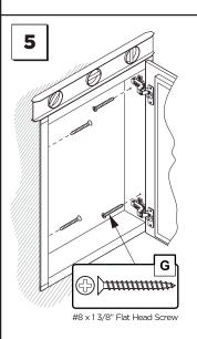
Level, then secure the cabinet with screws (**G**) through the mounting holes into the wall or the mounting studs.
