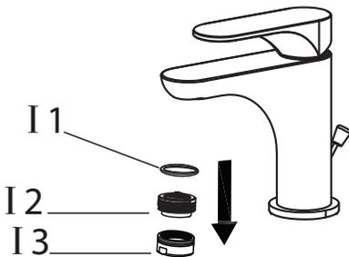
Remove aerator assembly (I). Loosen aerator cover (I 3) with adjustable wrench. Remove aerator (I 2) and aerator washer (I 1). Turn water on for 1 minute to remove any debris. Reassemble aerator assembly (I)
