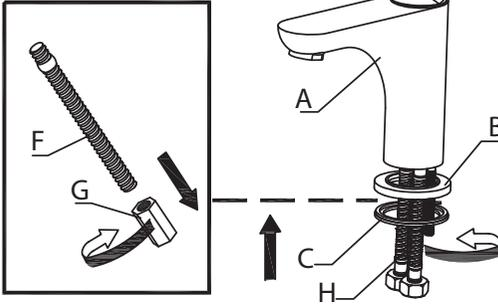
Remove faucet, mounting hardware, and waterlines from the box. Remove mounting nuts (G) from mounting screws (F). Place faucet body (A) on a soft cloth, spout facing up. Secure hot & cold waterlines (H) at the base of the faucet (HAND-TIGHTEN ONLY)
