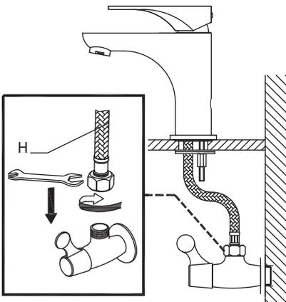
Thread hot & cold waterlines (H) onto angle stops and tighten with adjustable wrench until snug. Turn on angle stops and check for leaks (DO NOT TURN ON FAUCET)
