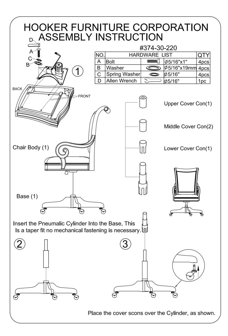
Place the chair body onto the cylinder. No mechanical fastening is necessary because this is a taper fit. Now sit in the chair. This will firmly secure the taper fit.
