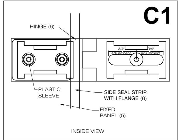
2. Screw the hinges (#6) to the fixed panel (#5) with the hex key (supplied).
