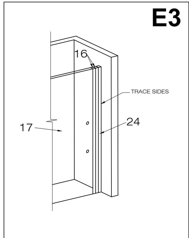
4. Open the door (#17) and remove the magnetic seal strip (#16) from the vertical rail (#24). Position the vertical rail (#24) along the wall where you marked, making sure the bottom rests on the floor. Mark holes on the wall for mounting screws.
