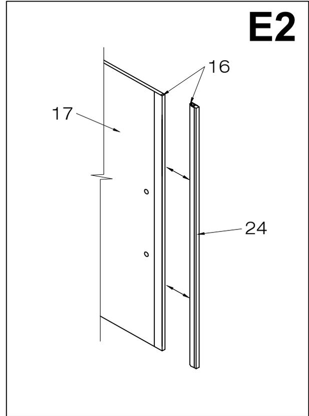
3. One person must hold the connection at the magnetic seal strips (#16) together and place the door in the closed position. The other person will mark the location of the vertical rail (#24) along the wall by tracing the sides.
