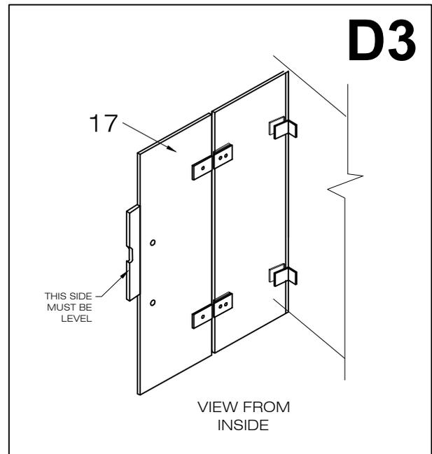
4. Clean the door (#17) glass surfaces where the magnetic seal strip (#16) is to be installed with rubbing alcohol. Place the magnetic seal strip (#16) to the door panel. The magnetic side should be facing the inside and the clear side be facing the outside. **⚠ Do not install the handle first, this is dangerous and may cause the glass to break.**
