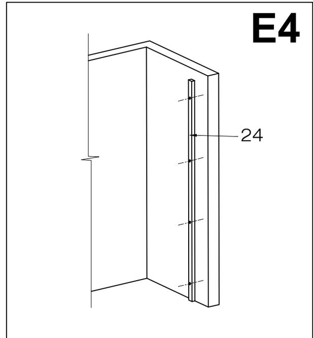
5. Remove the vertical rail (#24). Drill holes into the respective marks and insert green plastic anchors (#23) inside them.
