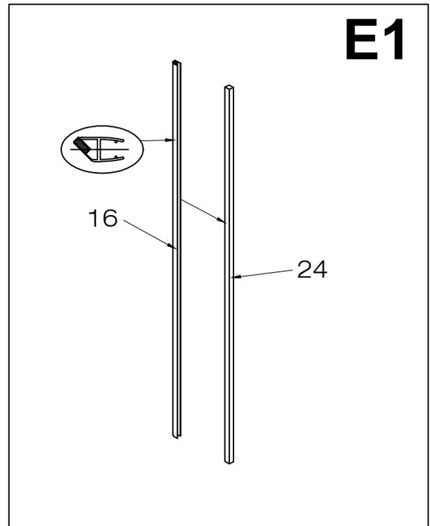
2. Connect the vertical rail (#24) to the door panel (#17) by the magnetic seal strips (#16).
