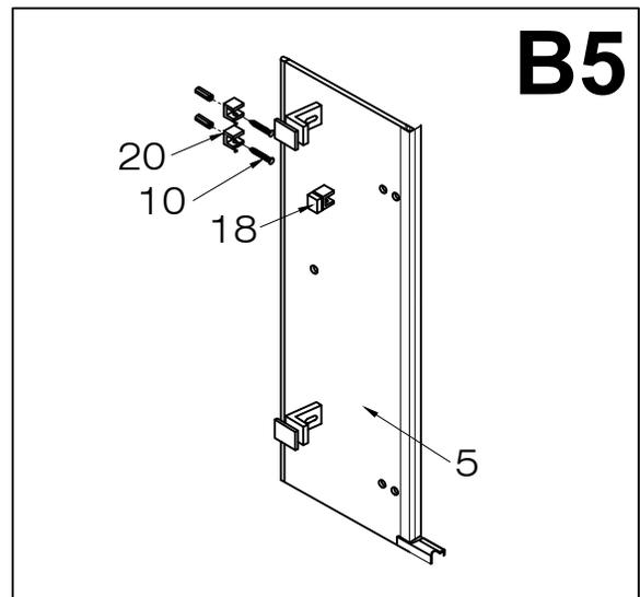
6. Slide the shelf glass (#19) into the three shelf glass holders (#18 and #20) and tighten the set screws from underneath. Repeat steps 1-6 to install the lower shelf glass.
