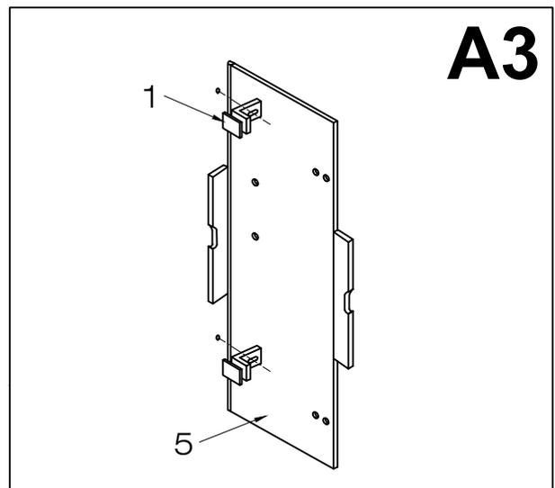
4. Remove the fixed panel and drill holes into the wall. Insert plastic anchors (#2) into the holes. **⚠ Not necessary if installing into studs. Studs are the preferred means of installation, anchors can pull out of the wall causing property damage and bodily harm. There is a 15mm adjustment built into the glass supports for minor modifications.**
