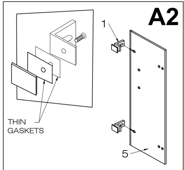
3. Mark holes on the wall for the mounting screws after leveling panel.
