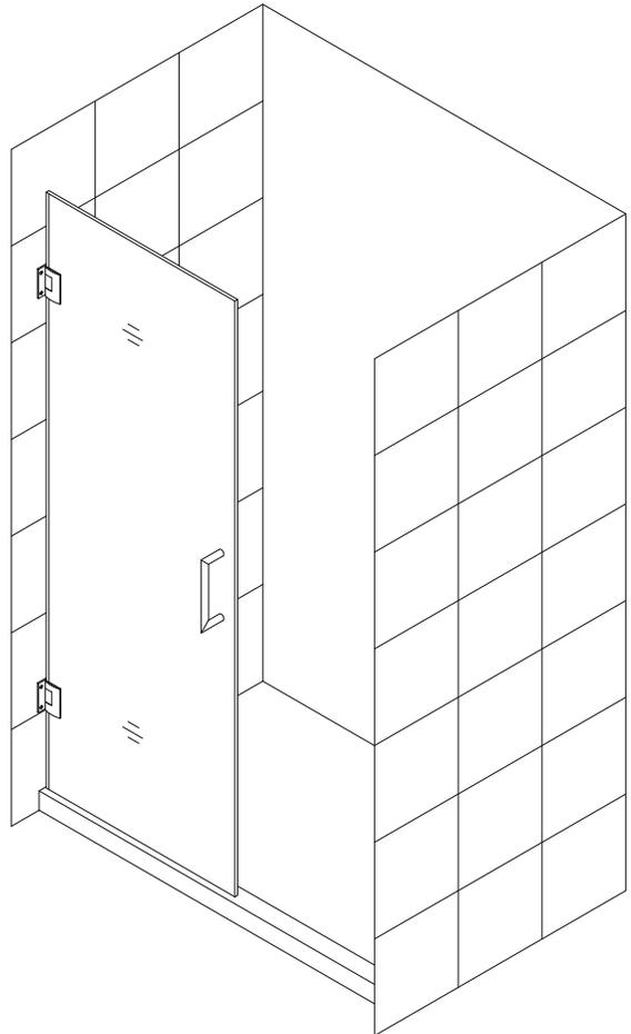
**NOTE:** The Unidoor hinge is factory set to over-close 8°. The following procedure is recommended to ensure proper alignment of the panel glass and door.
