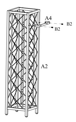
Assemble Connect Bar A4 to Back Frame A2 using Bolts B2.
