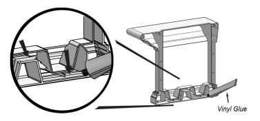
Identify the right and left end caps from the part list. Starting with only the Left End Cap, run a continuous bead of glue along the internal walls of the cap. Be generous with the glue to ensure a strong seal is formed between the panels and end cap.
