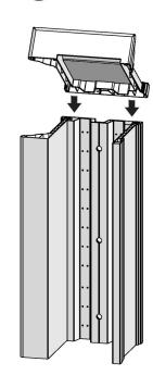
Stand the 3 panels on one end as shown on the left. Align the end cap at an angle and start by inserting the panels into the bottom portion of the end cap. You may need to wiggle the cap to get the panels to fit inside the guides. Work your way down by aligning the top portion of the panels with the end cap and rotate the cap downward as indicated by the arrows below. Once in place press firmly to ensure the cap is properly seated.
