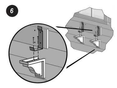
To install the optional decorative brackets align the holes with the wall mount brackets (decorative brackets are sold separately). Secure using the two screws provided with the decorative brackets. The molded vinyl brackets are decorative only so there is no need to over tighten the screws.
