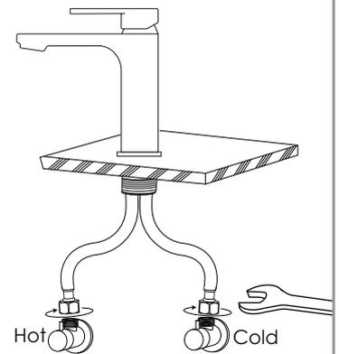
Connect hot and cold water lines to the inlet pipe and tighten with a wrench until snug. Do not over tight.
