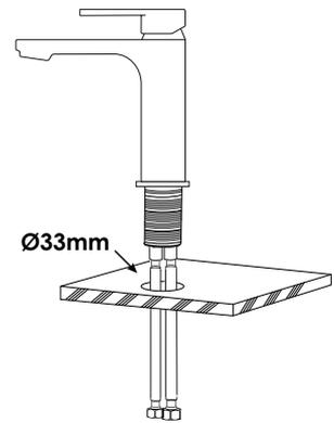
Ensure there is a Ø33mm through-hole on the counter. Position and insert faucet into faucet countertop hole.
