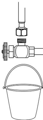
Before connecting supply hose, flush supply valves to clear any debris. Place a bucket underneath valves and run water for 5 to 10 seconds. Turn water off.
