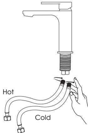
Install hot and cold water lines to the faucet. Hand tight hoses firmly.
