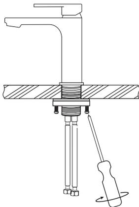
Tighten the mounting nut with the screws until faucet is firmly secure.
