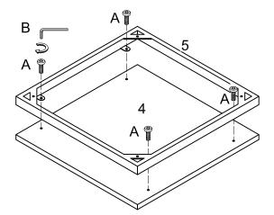
Secure wood panel (2) to frame (3) and wood panel (4) to frame (5) using bolts (A) as shown.
