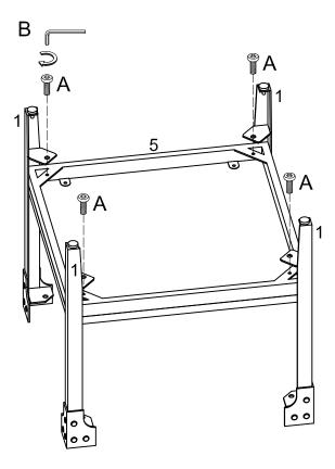
Attach legs (1) to frame (5) using bolts (A) as shown in the diagram.
