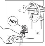
Attention: Screw the Drain Plug after the water reservoir is empty. Make sure the Drain Plug is screwed each time before use.
