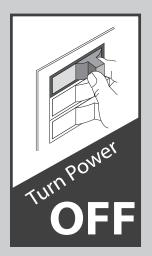
Be sure to turn off the power to the fan before performing any maintenance or relamping.
