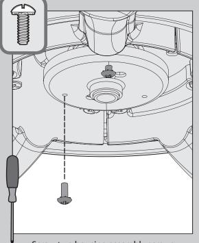
Screw two housing assembly screws
