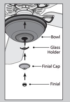
Press the bowl and glass holder flush against the metal plate. Thread the light pull chain through the hole in the center of the finial cap and thread the fan pull chain through the grommet hole in the side of the finial cap.
