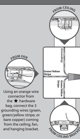
Note: To connect the wires, hold the bare metal leads together and place a wire connector over them, then twist clockwise until tight.
