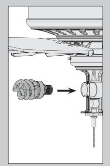
Install a bulb into each of the sockets. When necessary, replace with bulbs of the same wattage.
