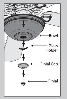
**Changing the bulbs** - Unscrew the finial and remove it from the threaded rod. Remove the finial cap and unscrew the globe keeper while supporting the globe with your other hand. Carefully remove the globe. Unscrew bulbs and replace with bulbs of same type and wattage. Reinstall the globe assembly.
