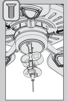
Insert three switch housing screws, found in the ≡ hardware bag.
