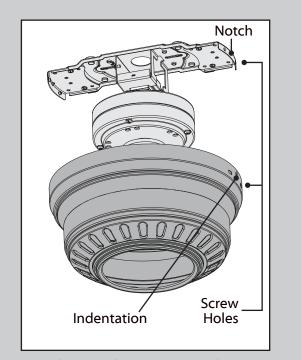
Raise the motor housing up over the motor and ceiling bracket. Turn the motor housing so the screw holes align and the indentation in the housing locks into place with the notch in the ceiling bracket. **The motor housing is not secured until the next step is complete. Do not leave unattended.**
