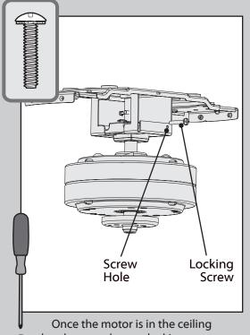
Solution Stracket, use the two locking screws found in the ★ hardware bag to secure the motor to the ceiling bracket.
