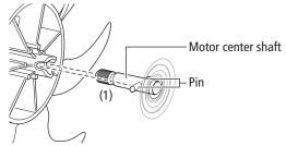
When the blades are assembled, align the blade center with the center of the motor shaft, and insert the blade into the motor shaft center. See Fig. ①.
