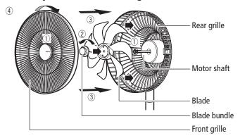
1. Align the blade to the motor shaft and install it. See Fig. ①.
