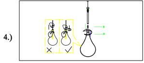
Step.4: Install G9 bulb (E) provided. Gently turn glass (F) onto socket (D) to secure.
