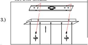
Step.3: Tighten screws (D) on the sides of the canopy (C) to secure the fixture.
