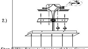
Step.2: Wire fixture to wires in outlet box. Green wire is for Ground.
