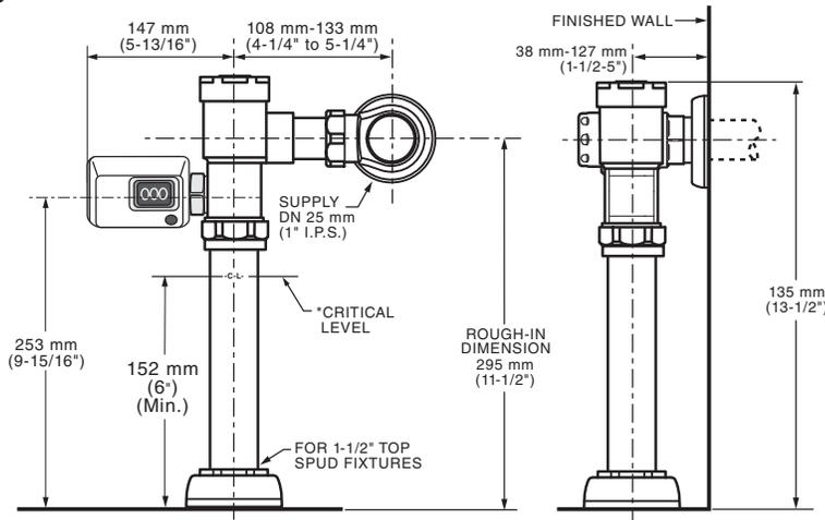
\*Note: The Critical Line (-C-L-) on Vacuum Breaker must typically be 6" (152mm) minimum above fixture. Consult Codes for details.
