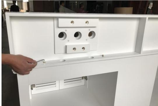
**Step 2:** Spacer blocks are preinstalled. Kohler valve (Model K-410-K-NA) is required for retrofit installation. Screw in the wood screw as shown through the back of mounting plate of the valve as shown. Connect with flex pipe as shown from the Kohler valve to the rough in valve. Your valve installation is now complete!!
