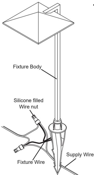
Note: Wire is to be protected by routing in close proximity to the Luminaire or fitting or next to a building structure such as a house or deck. Wiring should be buried a maximum of 6 inches (15.2cm) in order to connect to main supply wire. The main supply wire must have its length cut off within 6 inches (15.2cm) from a building structure, a Luminaire or fitting.
