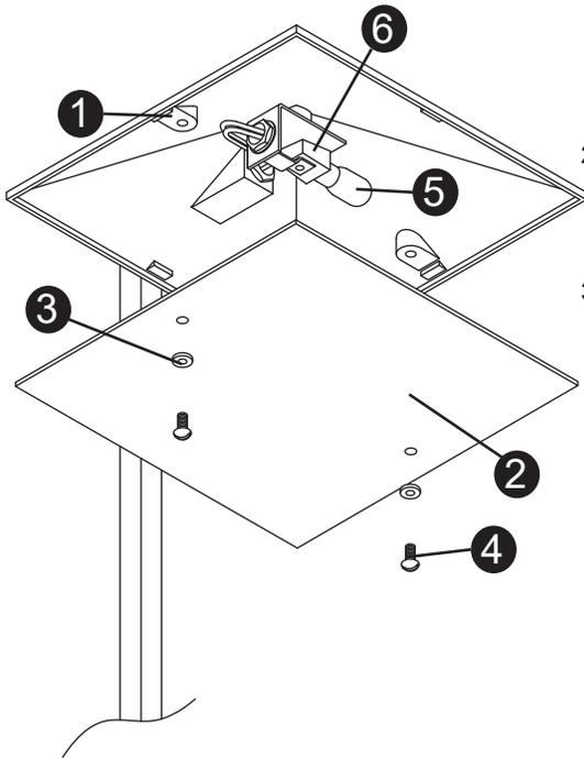
1. To install glass and lamp fixture, unscrew the two glass screws (4) from the screw notches (1).
