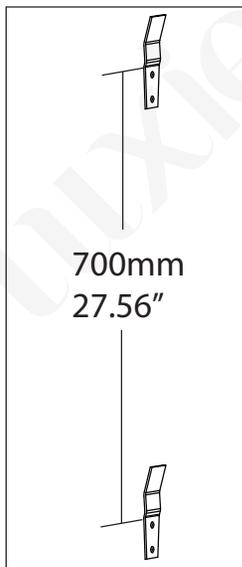
4. Lift the panel to determine the proper height and placement. It is recommended to aim the top horizontal body jet to the chest area for optimal showering experience. Mark the positions of the 2 brackets on the wall and set aside the panel.
