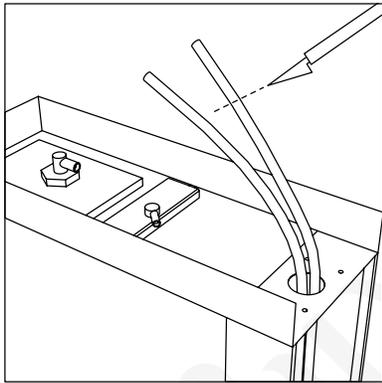
2. Trim off excess water supply hoses and attach to the spray head unit according to the hose labels and close the top cover.
