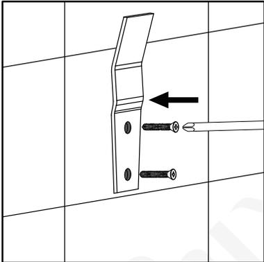
6. Secure the mounting brackets to the wall with the screws.
