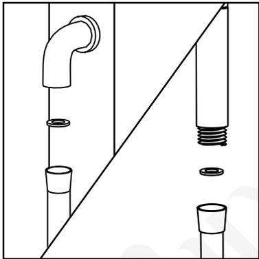
9. Connect hand shower hose to the main panel body and connect the hand shower wand to the hose. Make sure the silicon gaskets are seated properly to prevent water leak. The installation process is now complete.
