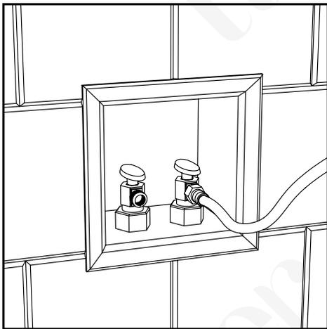
7. Apply thread sealant tape to the threading on the shut-off valves before connect both hot and cold water supply hoses to the valves.
