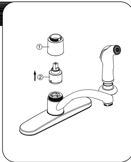
Loosen sleeve (1) by turning it counter-clockwise and lift out the cartridge (2). Remove the old cartridge and replace with the new cartridge. Replace sleeve and tighten. Reinstall the handle.
