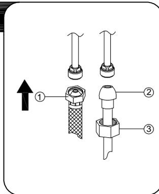
Make connections to water lines. Use 1/2" I.P.S. faucet connections (1) or use coupling nuts (3) with 3/8" O.D. ball-nose riser(2). Use wrenches to tighten connections. Do not overtighten.
