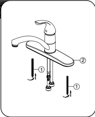
Shut off water supplies. Screw bolt (1) onto the escutcheon (2). If your model has a spray, proceed to step 2. If your model does not have a spray, skip to step 4.
