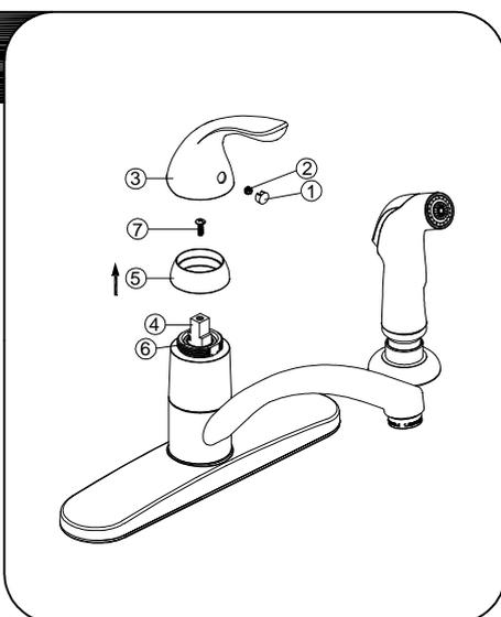
Shut off water supply. Remove set screw plug (1). With valves in "closed" position, unscrew set screw (2) and remove handle (3) from valve stem (4). Loosen the screw (7) from valve stem (4). Loosen the cap (5) from the sleeve (6).
