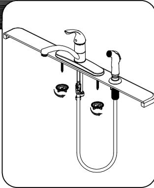
Place faucet in position on sink. From under sink, screw mounting nuts onto faucet. Tighten mounting nuts. Hand tighten only.
