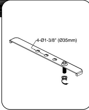
For models with spray ( fits 4 - hole sinks ): Insert spray support through far right - hand hole on sink. Screw hold - down nut onto shank and hand tighten.
