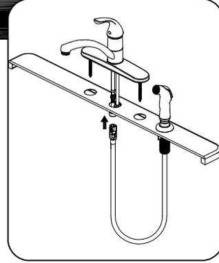
For models with spray: Insert spray hose down through the support and sink. Attach the spray hose to the connection beneath the faucet by aligning the tabs on quick connector. Push quick connector housing firmly upward and snap onto receiving tube tab. Pull down moderately to ensure connection has been made.
