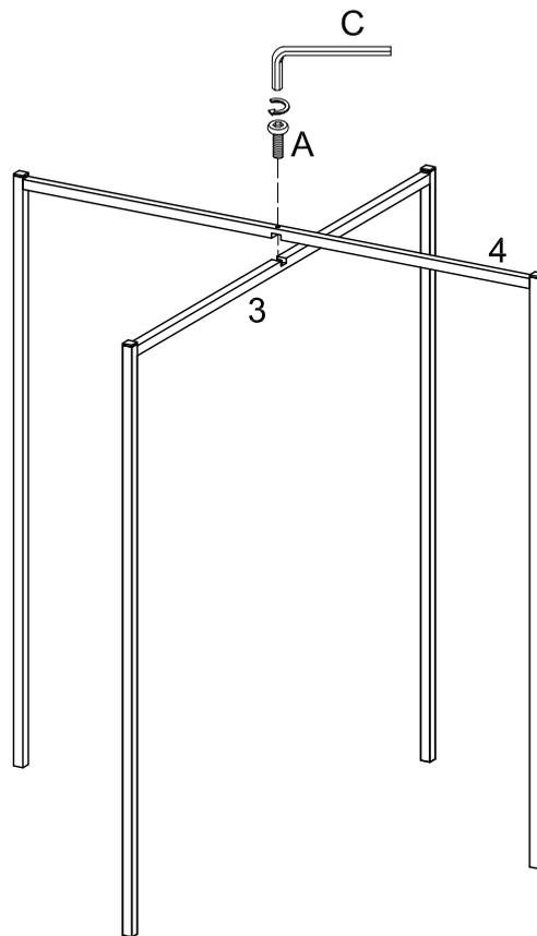
Use wrench (C), bolt (A) to secure the leg (3,4).
