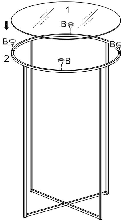
Insert the rubber suction cup (B), then place the glass (1) carefully on top of table top frame (2).
