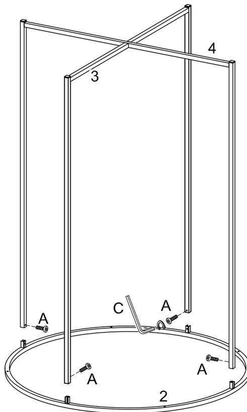
Use wrench (C), bolt (A) to secure the leg (3,4) to the table top frame (2).
