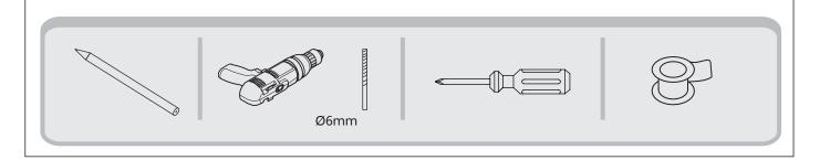
According to drilling drawing sheet to (B) mark the 3 drilling positions ①, then use the Ø6mm drill to drill holes on the wall according to the marked hole position.
