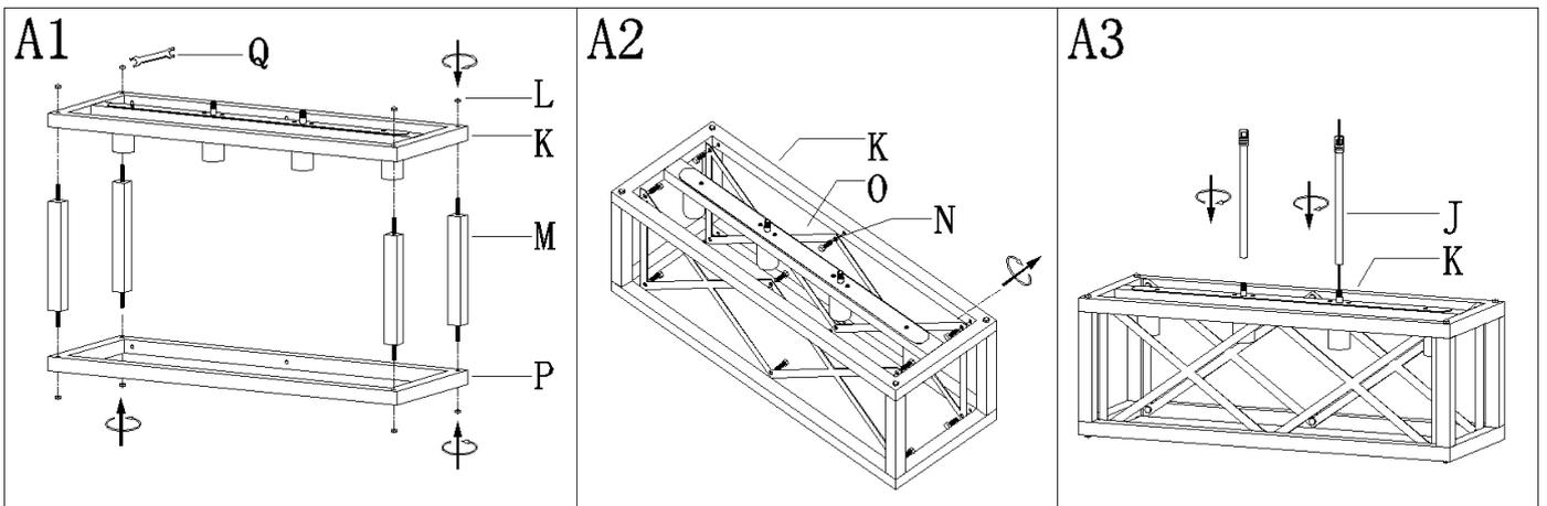
Step A1: Pass the batten (M) through the lower wooden frame (P) and secure with a hex nut (L).
