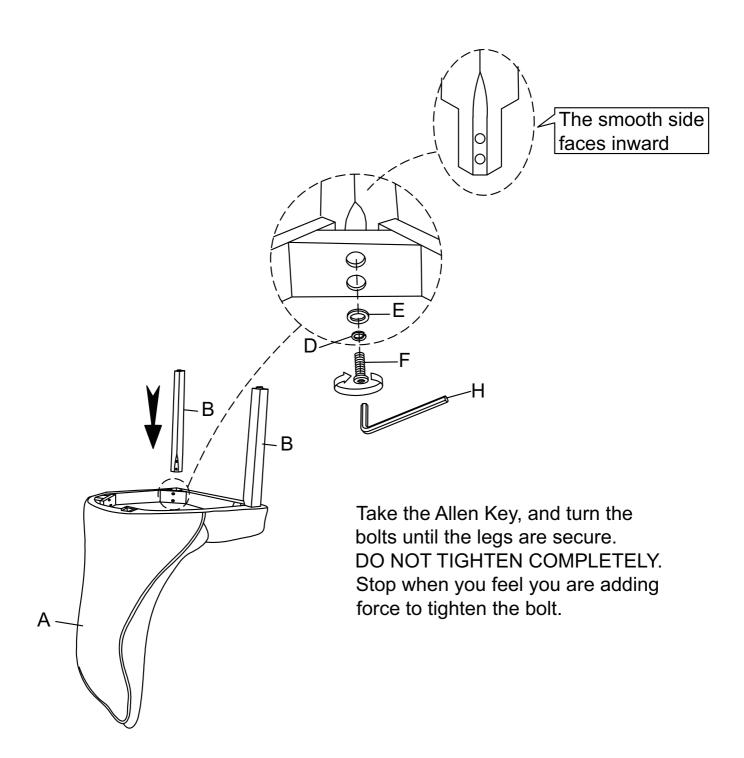
Attach the Back Leg (C) to Chair Body (A) with Lock Washer (D), Flat Washer (E) and Bolt (G) by Allen Key (H).
