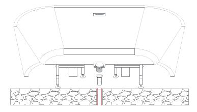
6. Flip the tub over and carefully set the tub into position with tail piece assembly to P-trap and connect to the drain.
