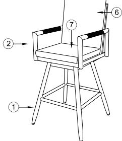
Step 2: Align the screw holes of the chair leg with the screw holes of the seat, insert flat washers(5) and screws(4) into each hole, once the screws are in place, tighten the screw until firmly attached with the wrench provided.
